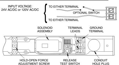
**HOLD OPEN FORCE ADJUSTMENT:** Locate hold-open adjustment screw in diagram above. For greater hold open force, insert socket screw key wrench (included in screwpack) and turn clockwise. To decrease amount of hold open force, turn screw counter-clockwise. Maximum of 4 turns.
